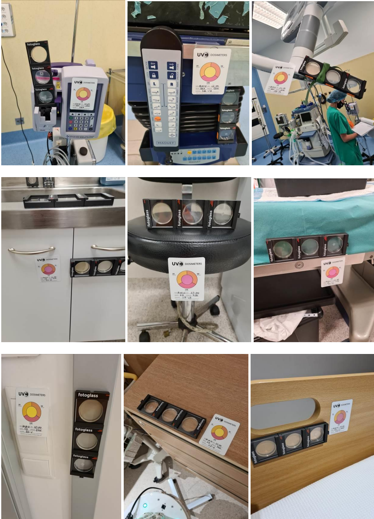
Installation of trio of biosensors and chemical dosimeters
