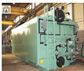
Cleaver Brooks Water Tube Boiler
